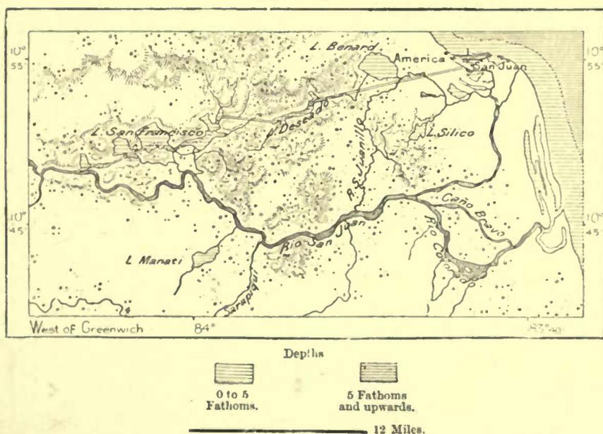
length of 170 miles, of which 140 of open navigation through the lake, and not more than 30 through ship canals. We are assured that vessels of the heaviest draught will take only 30 hours to pass from ocean to ocean, and that the cutting will admit 32 such vessels per day, or 11,680, of about 12,000,000 tons, a year.
