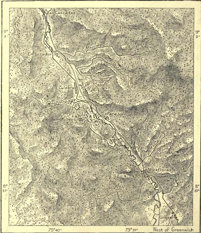
the valleys of the Chagres on the Atlantic and of the Rio Grande on the Pacific side. The crest of the range was to be crossed at Mount Culebra, either by a tunnel 130 feet high or by a tremendous open cutting. Reservoirs were to be constructed by means of dams to control the flood waters of the Chagres and its affluents, the displacement of matter being estimated at first at 1,645 millions of cubic feet, and afterwards at 2,520 millions, to allow for a tunnel nearly four miles long. But the
