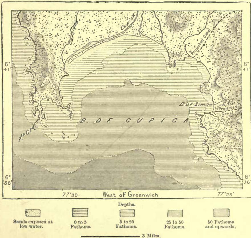
upper Tuyra and lower Atrato valleys. Wyse, however, has shown that this depression has no existence, and that the Tihule Pass, lowest of the range, is nearly 540 feet high. The canal, 140 miles long, would have required 22 locks, a tunnel 2,200 yards in length and much dredging about the Atrato estuary.
